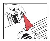
3. Remove Penetrant - When sufficient penetration time has been allowed, wipe the surface clean with a clean towel or cloth. Repeat if necessary. Some surfaces will require only wiping. In general, however, remove excess surface penetrant with clean cloths premoistened with cleaner/remover. DO NOT flush surface with cleaner/remover because this will impair sensitivity. Repeat this procedure with additional wiping until residual surface penetrant has been removed.
