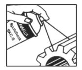
2. Apply Penetrant - Spray or brush the part or section to be inspected so that surface is covered with penetrant. If penetrant pulls back in droplets stop and clean part again. (Refer to Step 1). Allow penetrant to remain on the part from 10-30 minutes. Longer penetration times may be needed for locating extremely fine, tight discontinuities.
