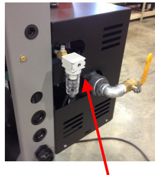
Incoming Air Connection 1/8" NPT Thread
