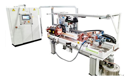
Our Universal SW stationary test benches are suitable for testing work pieces with clamping lengths from 1,200mm to 3,200mm. The clearance coil diameters of the basic units are 400 or 500mm. Universal benches can process test pieces with a maximum weight of 300kg (standard) or 1,000kg (optional).
